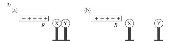
X and Y are two initially uncharged metal spheres on insulating stands, and they are in contact with each other. A positively charged rod *R* is brought close to X as shown in part (a) of the figure. Sphere Y is now moved away from X, as shown in part (b). What are the final charge states of X and Y?
