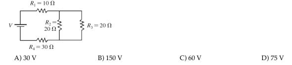
31) What is the potential drop from point A to point B for the circuit shown in the figure? The battery is ideal, and all the numbers are accurate to two significant figures.
